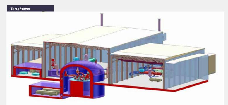
Molten Chloride Fast Reactor: In partnership with Southern Company, TerraPower will develop their Molten Chloride Fast Reactor (MCFR) technology. MCFR will utilize molten salt as 1) the dissolved fuel and 2) the heat transfer mechanism. The reactor will also operate under a fast neutron spectrum. The fast neutron spectrum is the primary difference between other MSR designs and TerraPower's MCFR. Using molten chloride salts will allow the reactor to operate under fast neutron spectrum conditions.
