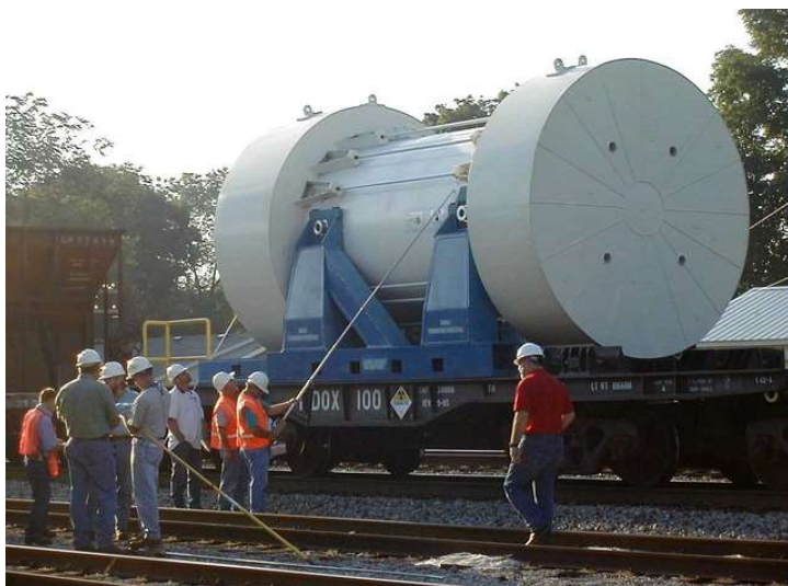
Figure 2: A railcar is used to transport a Type BF spent fuel package. Source: Idaho National Laboratory
